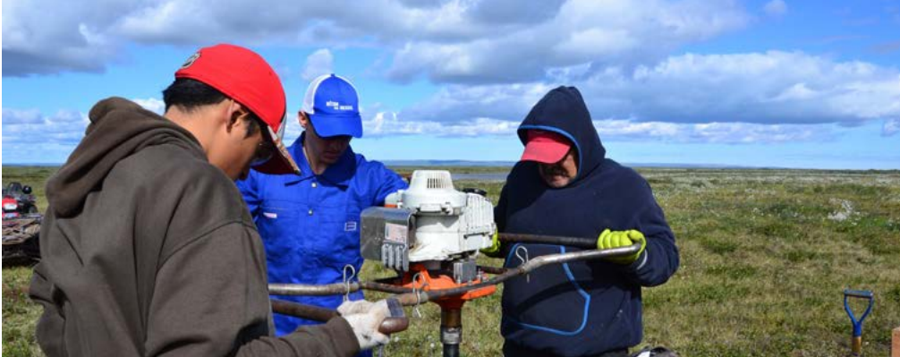
Taking core samples for community-driven research on permafrost degradation near Kugluktuk, Nunavut, Canada Credit: Polar Knowledge Canada
