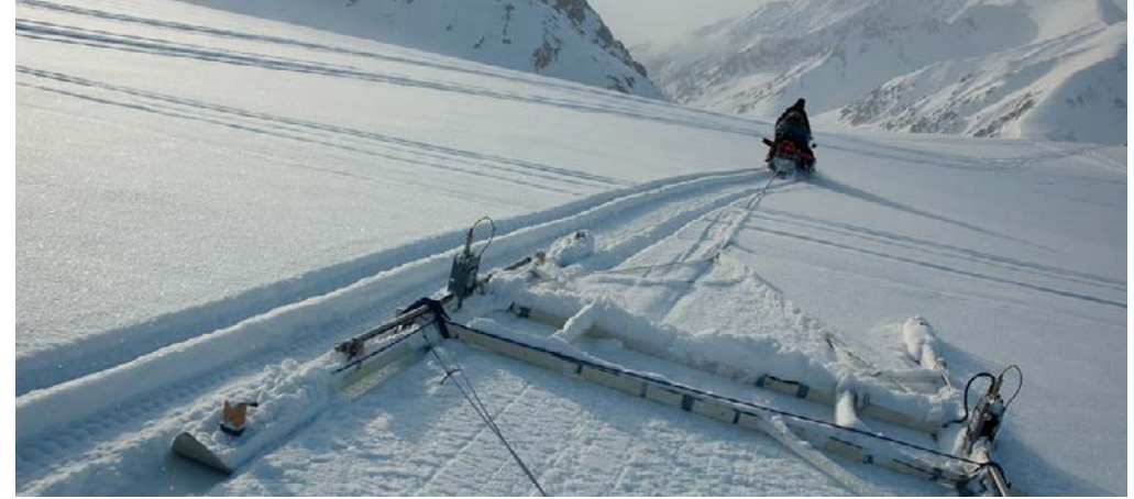
Measuring the ice thickness of a glacier in Greenland by ground penetrating radar Credit: G. Weyss
